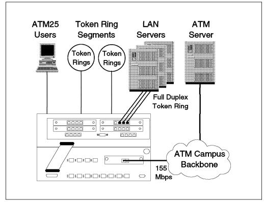
Figure 31. Relieving Ethernet Congestion with LAN Switching Module
